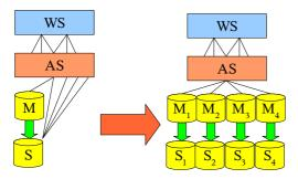
It should be considered that the splitting is done by the entity with the smallest possible interaction. Otherwise a lot of synchronization work has to be done between the concerned database nodes. It should also be considered that some data can or must be kept redundant (general
