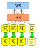
The disadvantage of this solution is, that you have to (keep) open at least 1 connection from each application server (AS) to each Master  $(M_n)$  and Slave  $(S_n)$  of each MySQL Replication cluster. So the limitation of this system is roughly:
